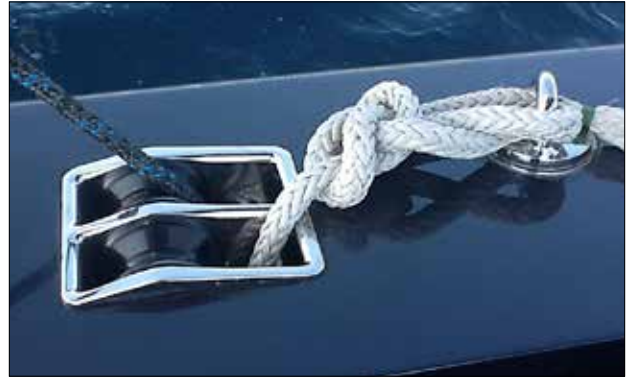
Above —A 3D model of the spinnaker sheet sheave gives a better understanding of what it will look like when installed. Right —The finished product in service.
